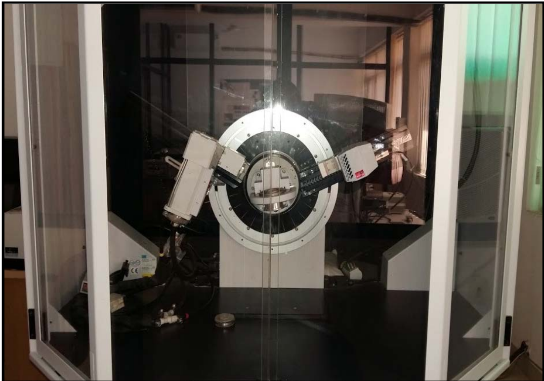
Figure 2.8: Photograph of the measuring chamber of the X-ray diffractometer
