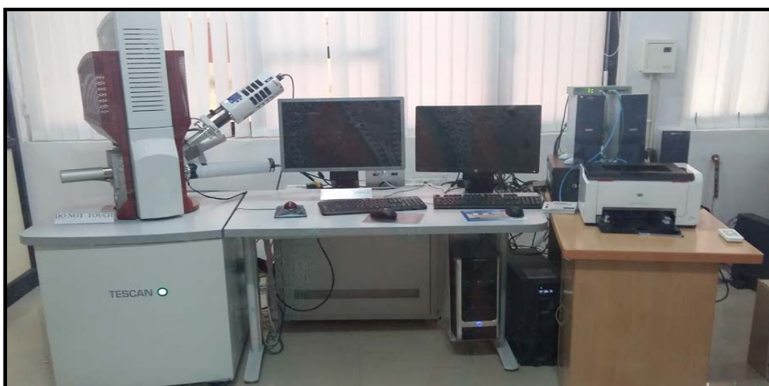
Figure 2.12: Photograph of TESCAN MIRA 3 FESEM instrument equipped with EDX
